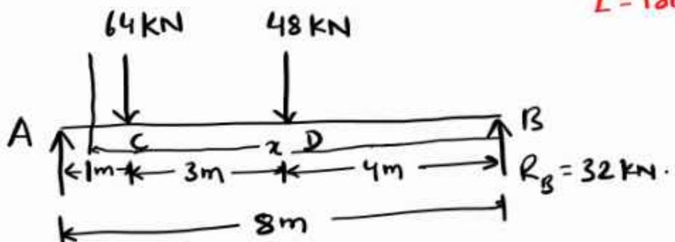
$$R_A = 80 \text{ kN}, R_B = 32 \text{ kN.}$$
