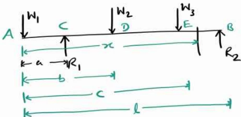
Consider a simply supported beam AB of length L as shown in figure. Taking A as origin and writing the expression for the bending moment.
