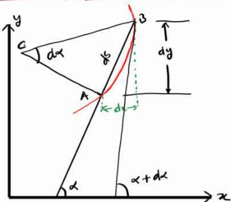
In given figure, a small portion of beam bent into an arc.
