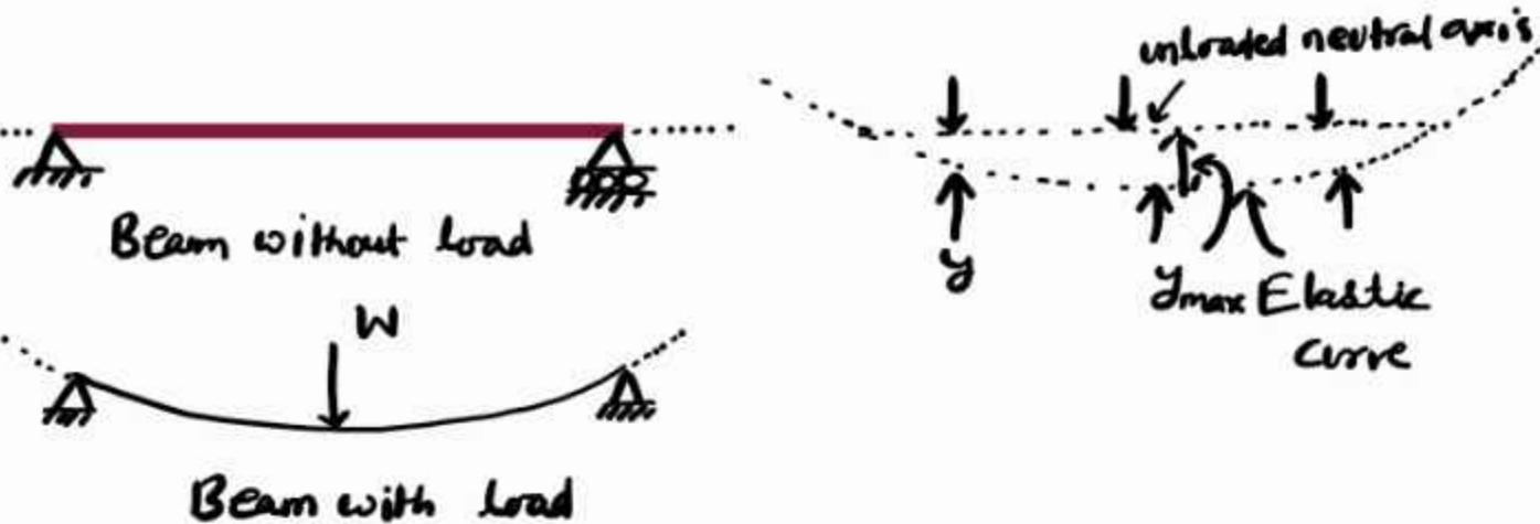
Under load neutral axis becomes a curved line and is called the elastic curve. The deflection 'y' is vertical distance between a point on the elastic curve and the unloaded neutral axis.
