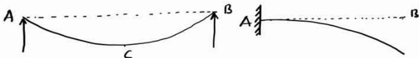
If considered origin at A, x is taken positive towards right and y positive upwards.
